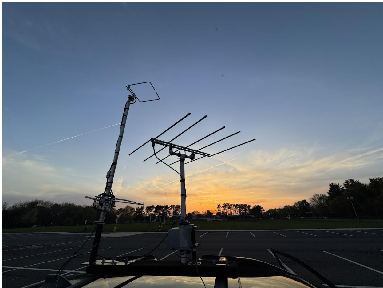
AA2SD/R testing a Elk Small Compact Log Periodic Beam on the Roof Rack with Stacked Halos during the twilight hour in Westampton NJ.
